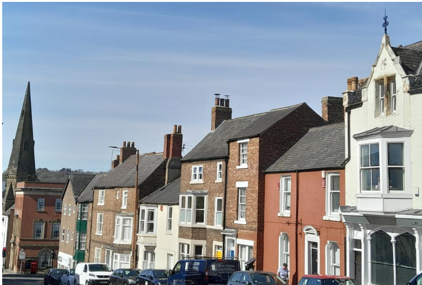
Fig 44 above. Claypath is a prime example of a fine historic roofscape with interest created by the different eaves and ridge levels, variation in roof pitches, and chimneys. The wall gabled dormer at No 61 and church spire are focal points.
